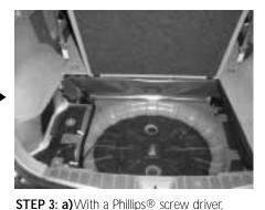
remove the driver's side cargo pocket. **b)** Unsnap the wiring harness that is running from front to back, on the floor.
